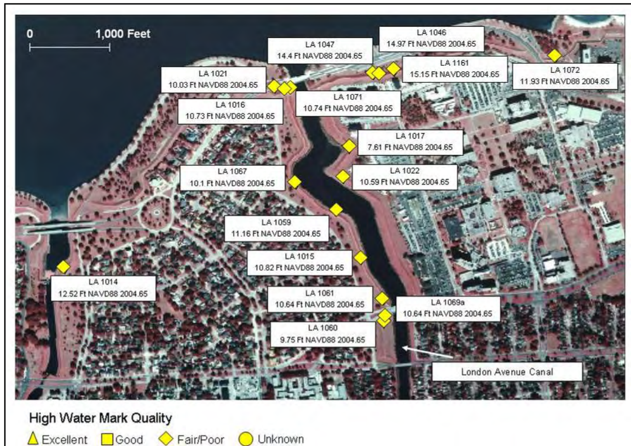
Figure 7. London Avenue Canal Entrance showing locations of HWMs and water elevation for each mark
