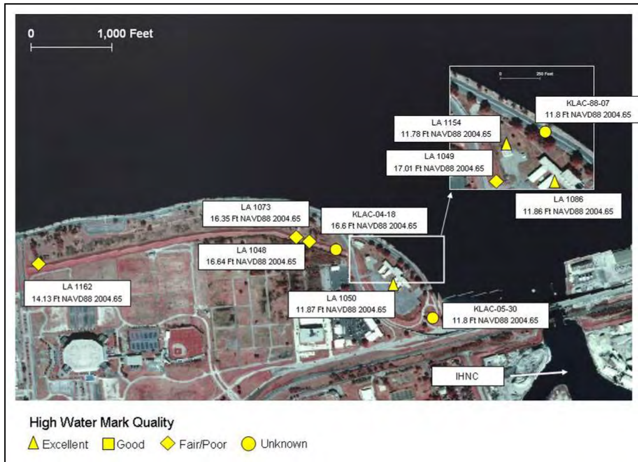
Figure 8. Lake Pontchartrain entrance to the IHNC, west side, showing locations of HWMs and water elevation for each mark
