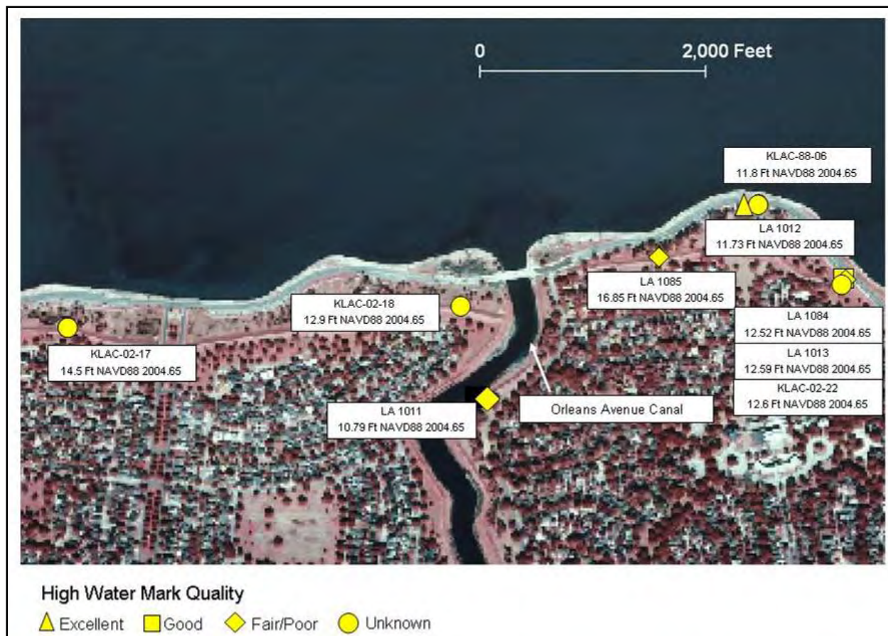
Figure 6. Orleans Avenue Canal Entrance showing locations of HWMs and water elevation for each mark
